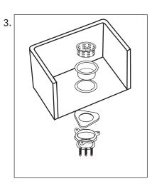
4. Screw in the 3 screws (not included) into the Mounting Ring.
