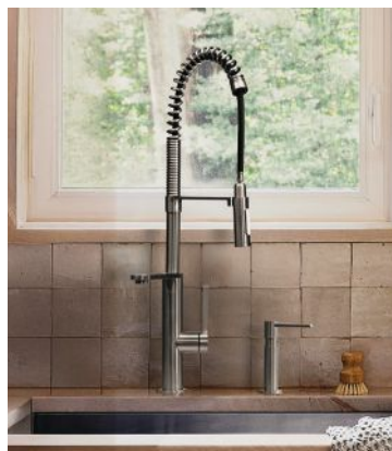
The K225 Faucet, part of Lenova's Design Edition Collection, offers both a pot filler and a pull-down dual-function spray head. The faucet features 360-degree rotation, magnetic docking, a ceramic valve cartridge and PVD coating. It is crafted from 304 stainless steel with zero lead content. lenovagroup.com
